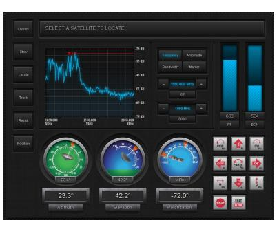
The RC4500-7200 Antenna Controller is a direct replacement for the Vertex/GD 7200 ACU. The RC4500-7200 can interface directly to a 7150 outdoor box, or can be used with an RCI designed outdoor unit.
