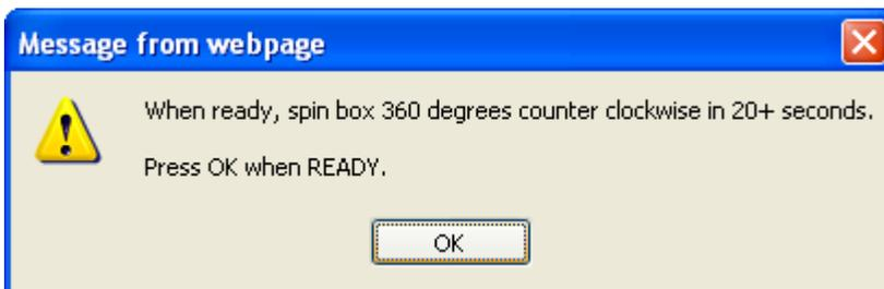
Step 9) Rotate the box 360 degrees counter-clockwise taking at least 20 seconds to complete the rotation. The unit should be kept as level as possible.
