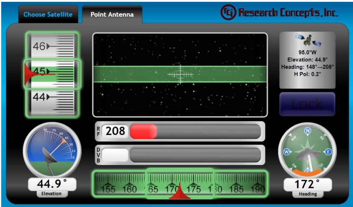
Step 4) Begin scanning across the target box by adjusting the antenna's heading until Source Lock (DVB, BCN – SBS2 Beacon, EXT - External) is achieved.
