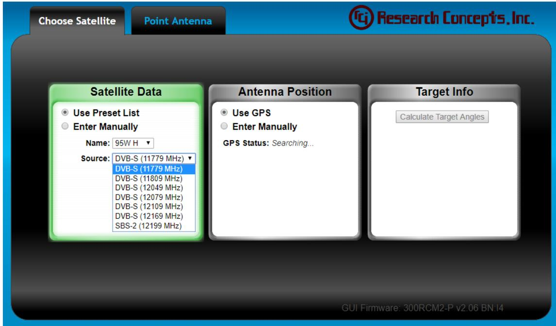
Step 4) Wait for the GPS receiver to achieve a valid lock. The GPS Status will change from “Searching...” to “GPS Ready” when the GPS receiver achieves a valid lock.
