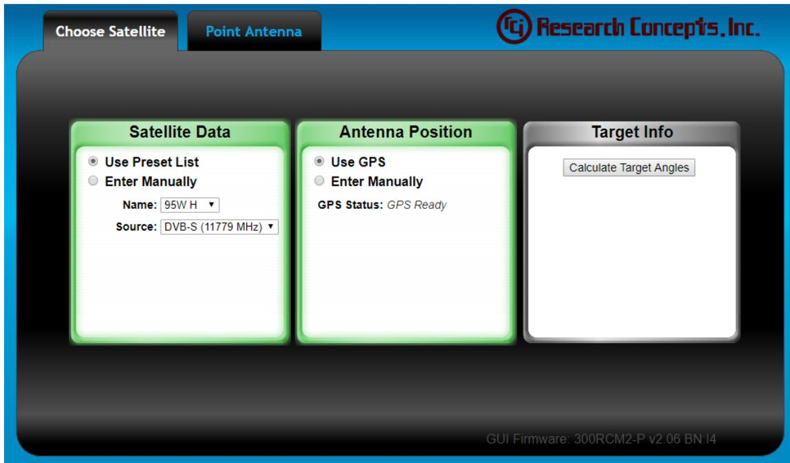
Step 5) Click the “Calculate Target Angles” button to calculate the target angles.
