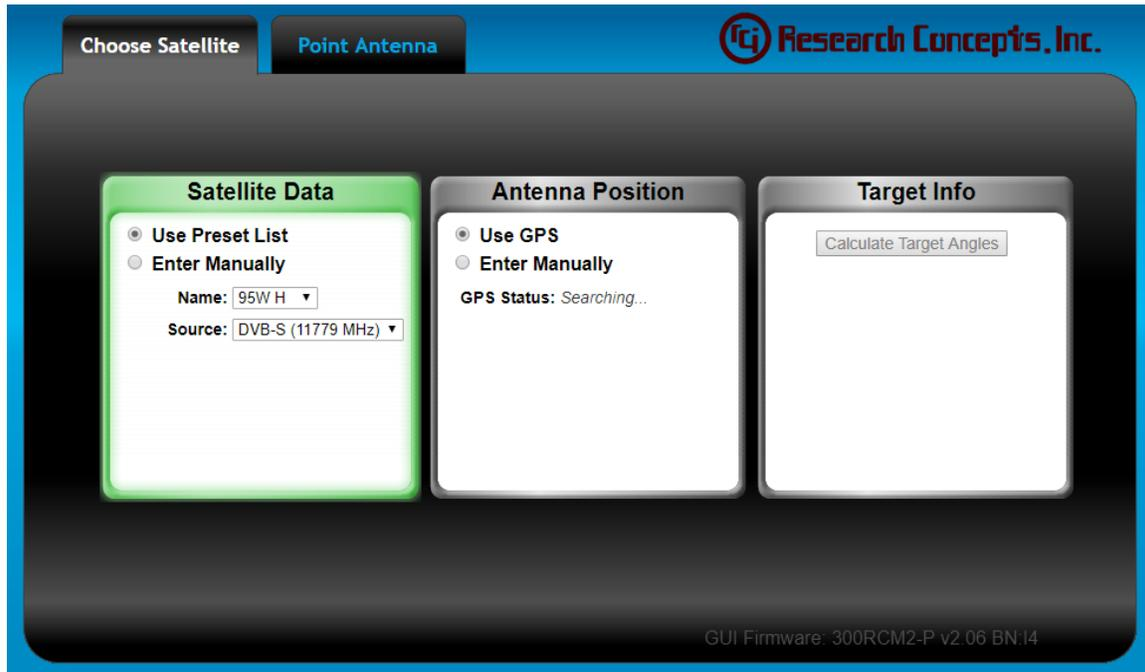
Step 2) Select the name of the target satellite by clicking on the “Name” drop down box.
