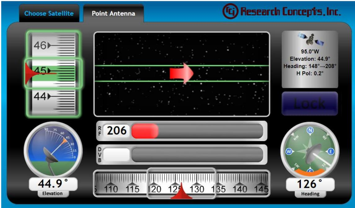
Step 3) Adjust the antenna's heading until the crosshair is displayed in the target box.
