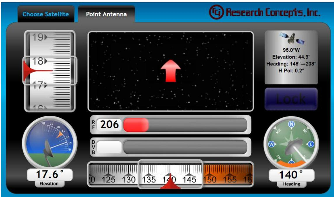
Step 2) Adjust the antenna's elevation until the target elevation is reached.
