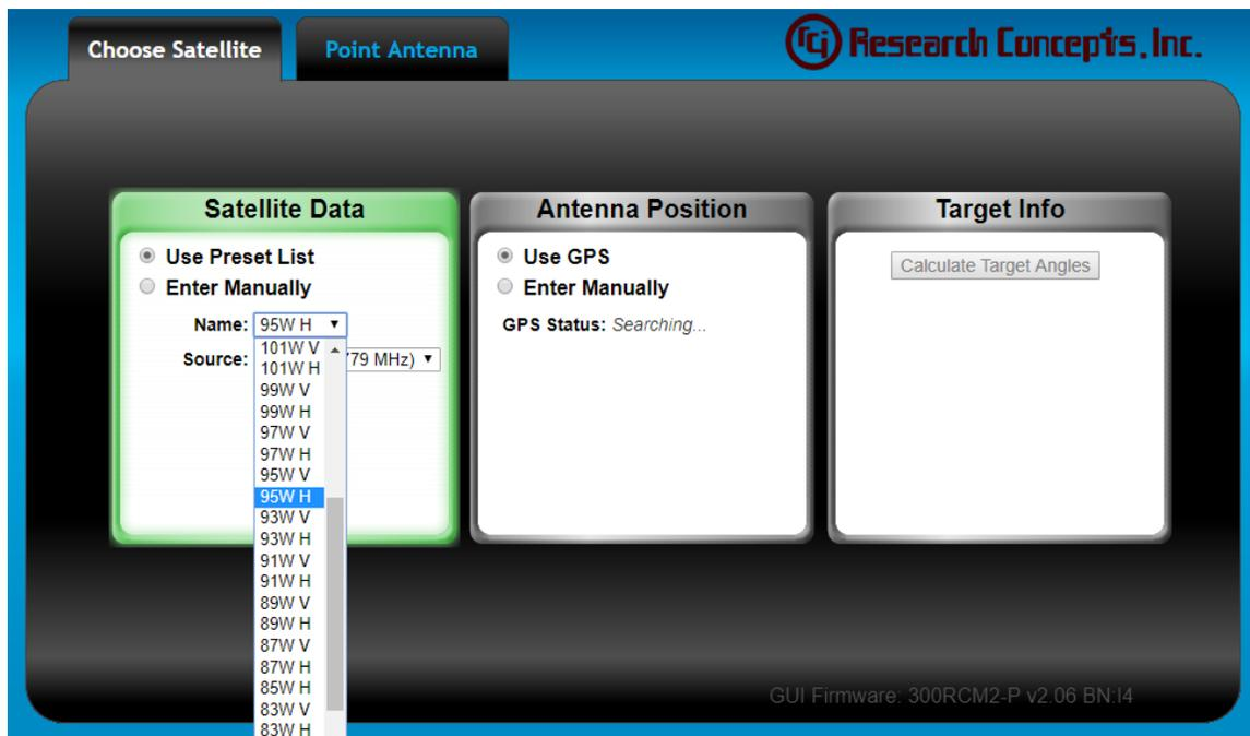
Step 3) Select the signal source and frequency of the signpost by clicking on the “Source” drop down box.
