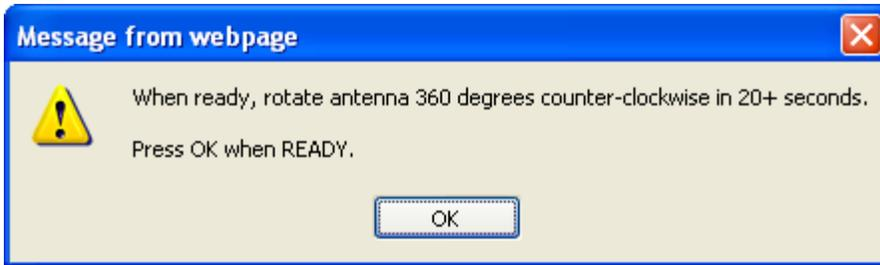
Step 8) Rotate the antenna 360 degrees counter-clockwise taking at least 20 seconds to complete the rotation. The antenna should be kept as level as possible.
