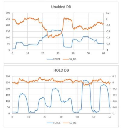
Measured performance using a Ku-Band antenna monitoring Satellite Beacon Signal Strength (Right-Scale in dB). The Antenna was pulled with a varying amount of force (Left-Scale, Ibs.).
