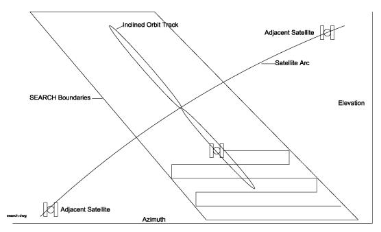
is calculated based on the satellite inclination angle specified by the user when the track is initiated from SETUP mode. The width (or short dimension) of the parallelogram is specified by the *Search Width* parameter entered via CONFIG mode. The *Search Width* has a range of values of 1 to 10, with 1 specifying the narrowest search window and 10 specifying the widest window. The default value of 3 is adequate for most situations.
