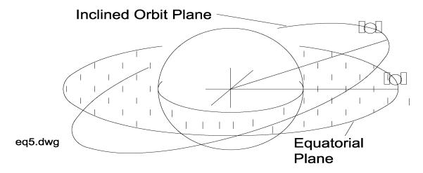
geostationary satellite appears fixed in space, the apparent position of a satellite in an inclined orbit varies with time.
