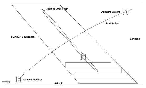
The automatic search may be disabled via the Search Enable CONFIG mode item. If the automatic search is disabled, the user is prompted to manually position the antenna on the satellite.
