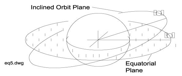
motion of the satellite is periodic, which means that the figure eight pattern repeats itself. The period of the motion is 23 hours, 56 minutes, and 4 seconds. The angle subtended by the figure eight pattern from North to South (i.e. height of the figure '8') is twice the inclination angle. The angle subtended by the figure eight pattern from East to West (i.e. width of the figure '8') is approximately the inclination angle (in degrees) squared and divided by 115.
