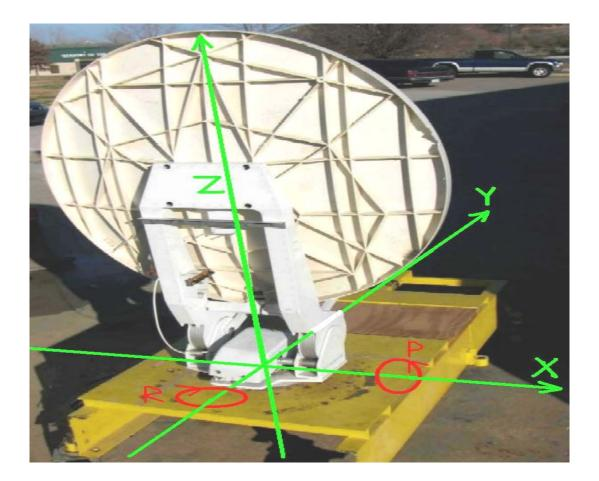
The TAC provides six possible orientations for maximum flexibility. The six orientations may be thought of as the six sides of a cube surrounding the antenna platform. A description of the cube face is given to each orientation as a way to help describe it.
