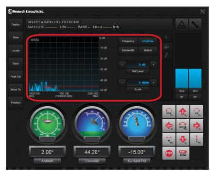
The Spectrum Analyzer functional window consists of the spectrum display on the left side and spectrum analyzer controls on the right side.
