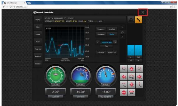
To configure the SBS spectrum analyzer, select the CONFIG tools button in the upper right corner, or add "/config" to the IP address.
