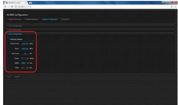
The SBS spectrum Analyzer initial settings can be set and "Save"d on this page. The factory default values are shown. An IP reset of the Web Server PCB of the RC4000 will return the values to those shown.
