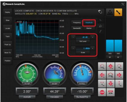
The Amplitude control allows the Reference Level and Vertical Scale (dB/division) to be adjusted. Again, both controls are incremented/ decremented via the + - buttons. The allowable values for Scale are 1, 2, 5, and 10 dB per division. The Reference Level increments by 5dB steps and can also be direct entered. The allowable Reference Level range is -70 to 0dB.
