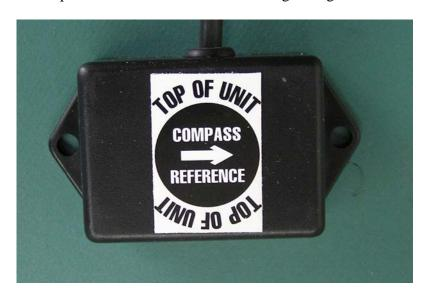
Next a compass box in the vertical mounting orientation is shown:
