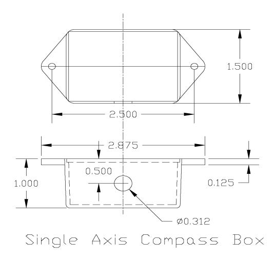
The compass box provides 2 mounting holes on end mounting flanges. The part number scheme for the compass is:
