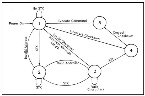
Figure 2 – SA Bus Protocol State Diagram
