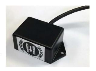
The Research Concepts three-axis compass is a low-cost alternative to the fluxgate compass that provides antenna heading, pitch and roll as well as calibration for magnetic distortions. A very small form factor PCB allows the compass to be conveniently housed in a small enclosure that may be installed on an antenna in one of six different orientations.
