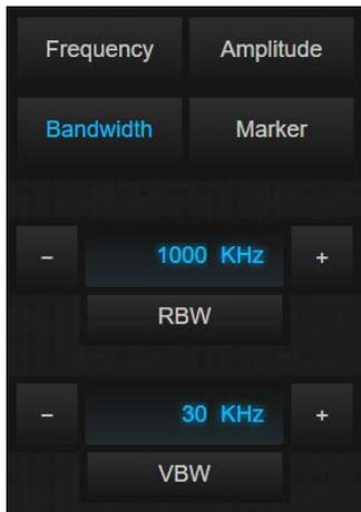
The Bandwidth Controls allows the Resolution Bandwidth (RBW) and Video Bandwidth (VBW) to be seen. The Resolution Bandwidth can be adjusted to:
