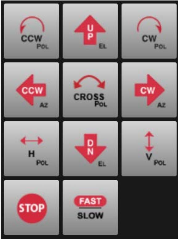
The bottom right side of the main page provides a keypad for manual jog control of the antenna. The keys provide the ability to jog the antenna in azimuth, elevation, and polarization. It also provides the ability to move to the preset H and V positions, as well as providing the ability to move the feed a preset 90° to cross pol.
