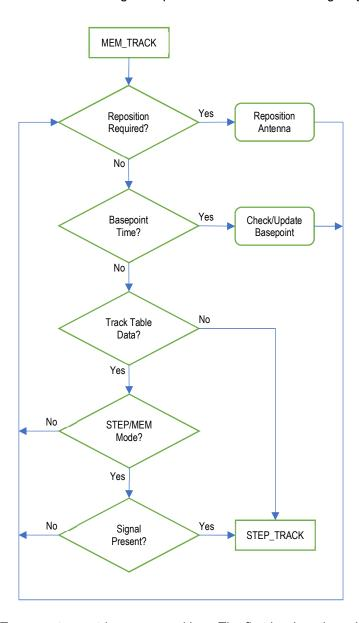
Two events can trigger a reposition. The first is when the calculated antenna pointing error exceeds the maximum tracking error (Reposition Required). The second is when the current sidereal time reaches one of the 48 track table entries (Basepoint Time).
