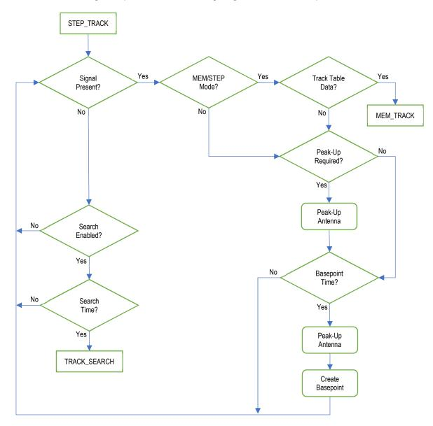
Two events can trigger a peak-up. The first is when the calculated antenna pointing error exceeds the maximum tracking error (Peak-Up Required). The second is when the current sidereal time reaches one of the 48 track table entries (Basepoint Time).
