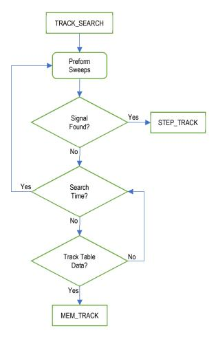
The ACU will sweep the antenna in a serpentine-shaped pattern over the region where it has calculated the satellite will be found. The extent of the search region is based on the antenna latitude/longitude, the satellite longitude/inclination, the antenna beamwidth, and the Search Width configuration item. In most cases, the search region is shaped like a parallelogram.
