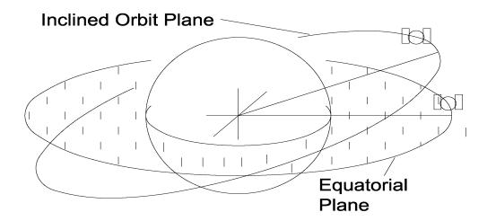
Whereas a geostationary satellite appears fixed in space, the apparent position of a satellite in an inclined orbit varies. If viewed by an observer located at the center of the earth, the motion of an inclined orbit satellite would be a figure eight centered on the earth's equatorial plane with a total height of twice the inclination angle.
