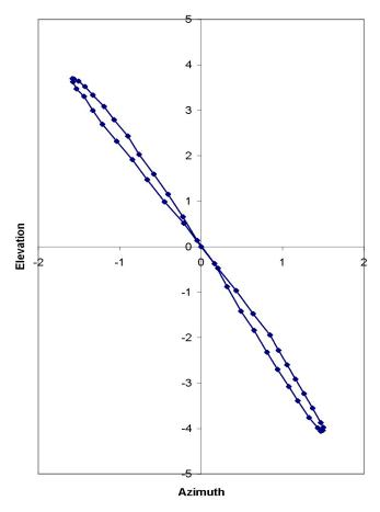
The motion of the satellite is periodic – the figure eight repeats itself every 23 hours, 56 minutes, and 4 seconds. This period is referred to as a sidereal day, or the time it takes the earth to complete exactly one revolution.
