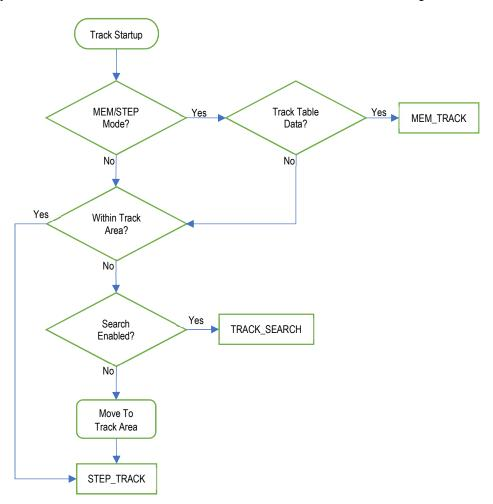
If a move into the track area is required, the ACU will first scan forward through the track table looking for an available basepoint. If a basepoint is found, the ACU will move to that position. If no basepoint is found, the ACU will move to the nominal position on the "arc" of satellites. Either of these positions should be a point where the satellite will eventually arrive.
