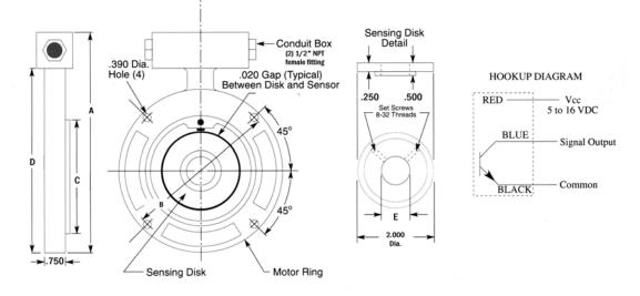
NOTE: To interface sensor to controller, use a shielded triple (18-22 AWG) with bare drain wire, such as Belden 8772.
