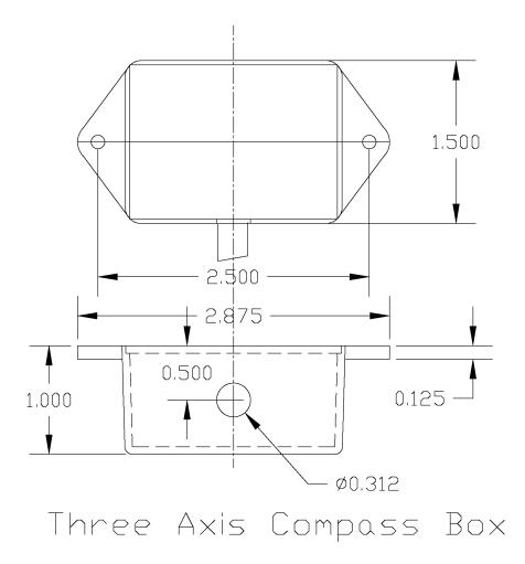
The TAC box provides 2 mounting holes on end mounting flanges. The standard part number for the compass is: FP\_CMPOS01 which includes a 42 ft. unterminated cable. Contact RCI for other cable length or connectorization options.
