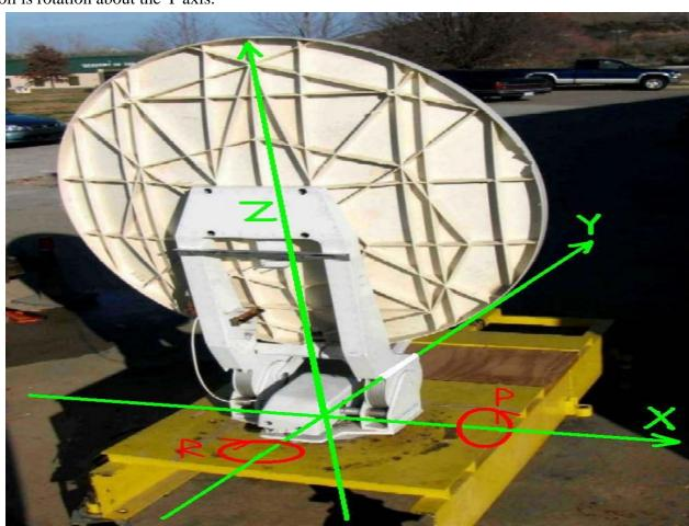
To correctly estimate antenna heading and to properly sense platform tilt, the TAC must be placed orthogonal to the antenna platform and must be calibrated while the platform is level.
