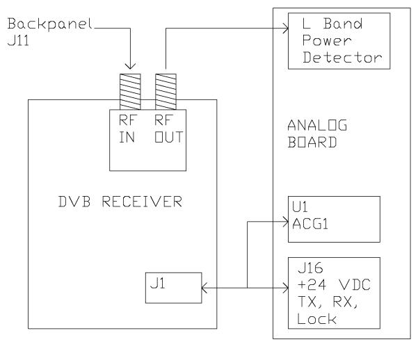
Power and serial communications will be mechanized via a cable between the DVB's J1 connector and the J16 connector on the analog board.
