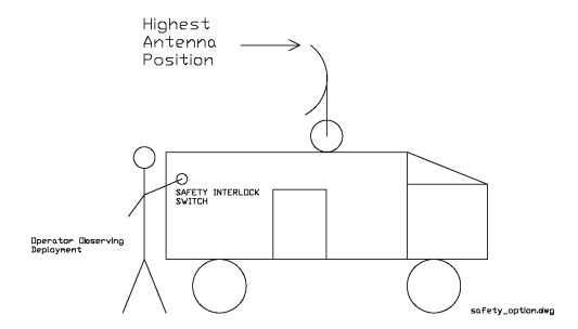
NOTE: this feature allows initial confirmation of safe antenna position after the powering up of the RC3000 antenna control unit. Another potential safety issue is that of vehicle movement with the antenna raised. The antenna integrator must mechanize an "antenna stow/vehicle interlock" in order to assure that the vehicle is not moved into dangerous obstacles while the antenna is not stowed.
