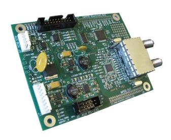
RC3000DVB is an internal DVB receiver card that is fully integrated into the RC3000 Architecture. The Satellite Locate Feature of the RC3000 product is further enhanced by the DVB Signal Scan Feature.
