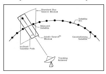
If the antenna beamwidth is larger than the width of the figure 8, it can track the satellite with single-axis, declination motion. An 11.5m C-band or an 3.8m Ku-band antenna would have a 3dB beamwidths of about 0.6 degree. Properly aligned, these antennas could track the satellite with less than 3dB error.
