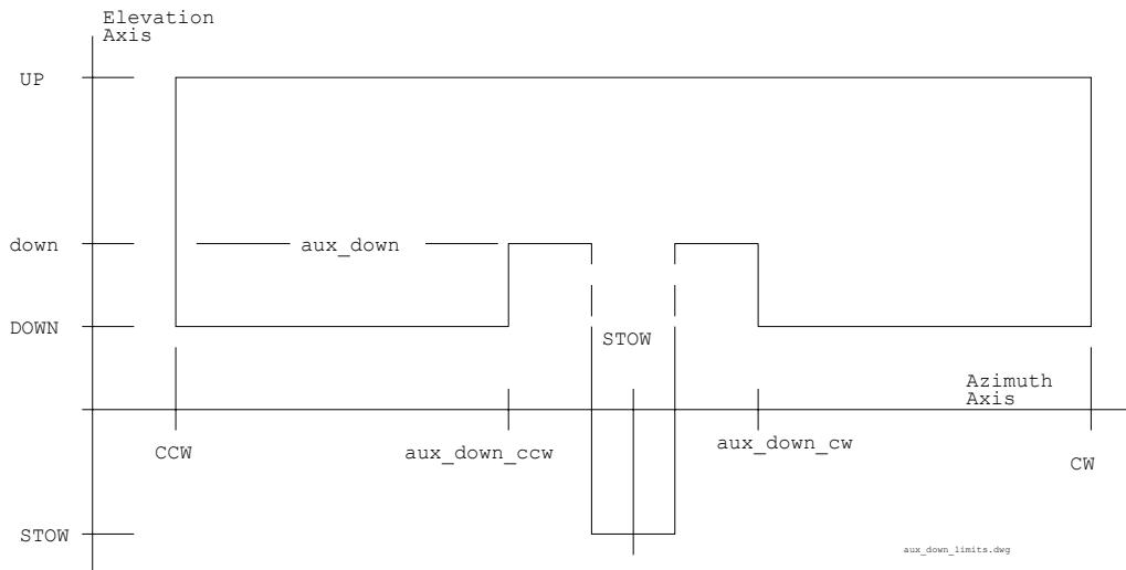
When outside of the auxiliary region, the down limit is defined by the hardware elevation down limit switch. The auxiliary down region allows the hardware limit switch to be set lower than normal.
