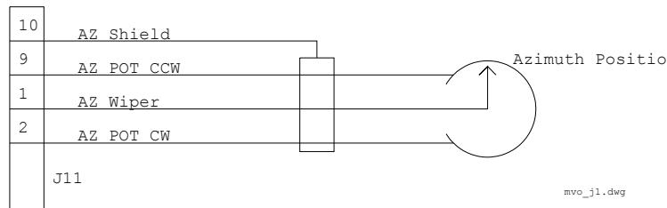
NOTE: J11 is used for the azimuth resolver on the R5 version.
