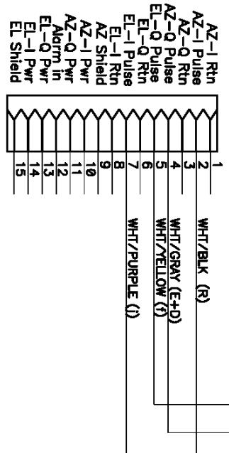
attach to PCB mounted DB-15F with
