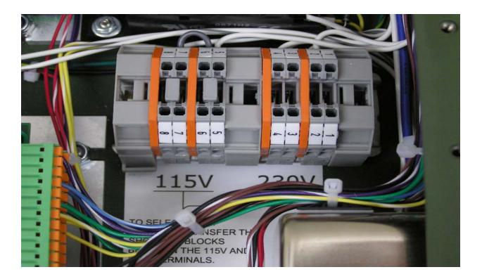
The second modification involves placing two switches on the motor drive module in their correct positions. The following picture shows the switches in the 115 VAC position (both outward).
