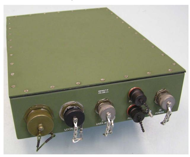
The chassis of the RC4000 consists of a frame with a floor, and separate end panels and lid.
