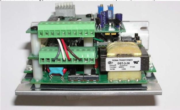
To place the drive module in the 230 position, move both switches to their inward position.
