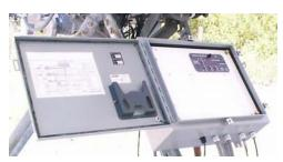
Enjoy the High resolution and accuracy of resolvers as position senors on antennas equipped with 36VDC linear actuators. Allows the use of the RC2500 with inexpensive antenna systems.
