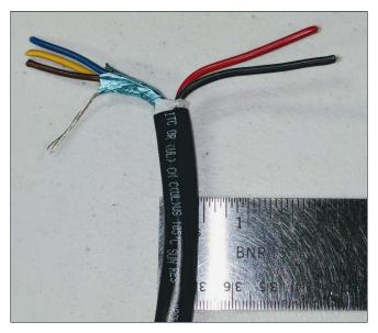
The above three wires are contained in a 100% insulated foil shield with a contacting 18 AWG bare drain wire.
